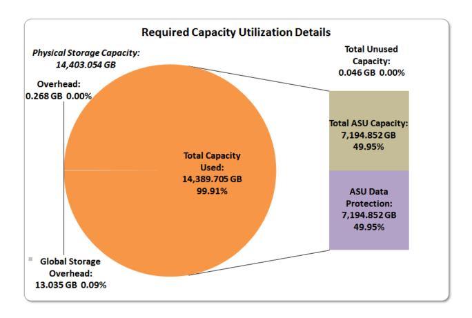
The Tested Storage Configuration (TSC) must be configured so that there is either no more than 1 GB of Unused Storage (100% utilization) or that the sum of Total ASU Capacity and storage required for data protection equals 50% (+-1 GiB) of the Physical Storage Capacity.
