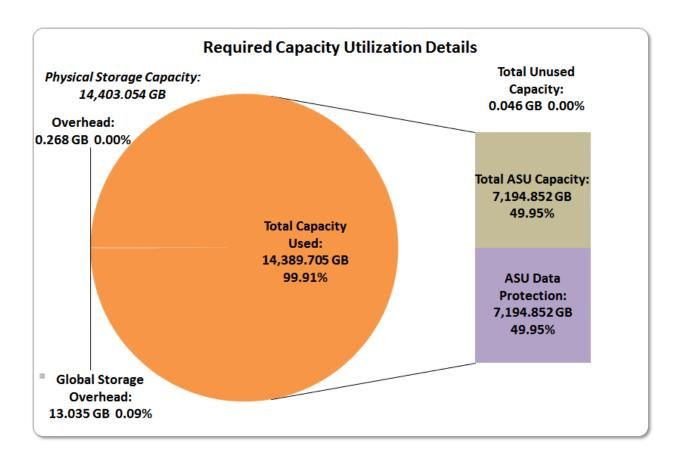
The Tested Storage Configuration (TSC) must be configured so that there is either no Unused Storage or that the sum of Total ASU Capacity and storage required for data protection equals 50% (+-1 GiB) of the Physical Storage Capacity.
