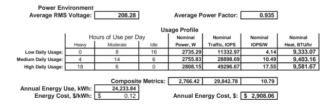
The above usage profile describes conditions in environments that respectively impose light ("low"), moderate ("medium"), and extensive ("high") demands on the Tested Storage Configuration (TSC).
