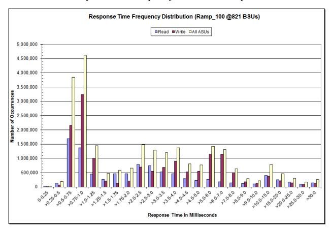
**IOPS Test Run – Response Time Frequency Distribution Graph**
