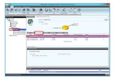
b. Right-click on the disk (**Name** column) and select **Add Mirror Disk** and select a disk of the same type to mirror to.
