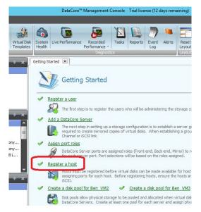
b. Enter the **Computer name** from the table below, Set **Operating System** to Microsoft Windows, Select **Multipath Enabled**, and set **Preferred server** to All. Then use the table below to chose the four proper WWNs of the FC initiator ports for the Computer named and then click the **Register** button.
