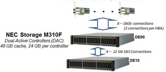
1 - M310F Dual Controller Disk Array Unit (includes Disk Enclosure DE00)
