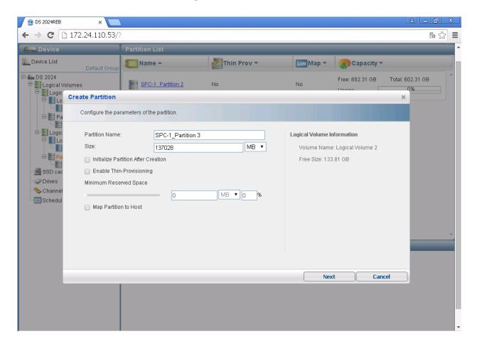
Step 12: As was done for Slot A (Controller A) in <a href="Step 7">Step 7</a> and <a href="Step 8">Step 8</a>, map partitions, SPC-1\_Partition-3, with selections of Customize the host LUN mapping configurations, Fibre 16.0 Gbps and Channel 4/Channel 5 for Slot B (Controller B). Then click OK after mapping each partition.
