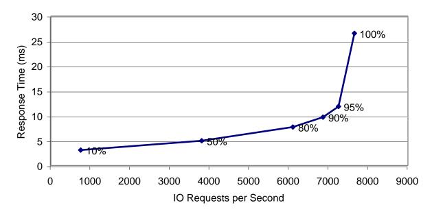
Ramp Phase Response Time / Throughput Curve
