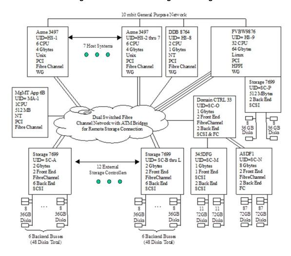
Figure 10-1 BC/TSC Configuration Diagram
